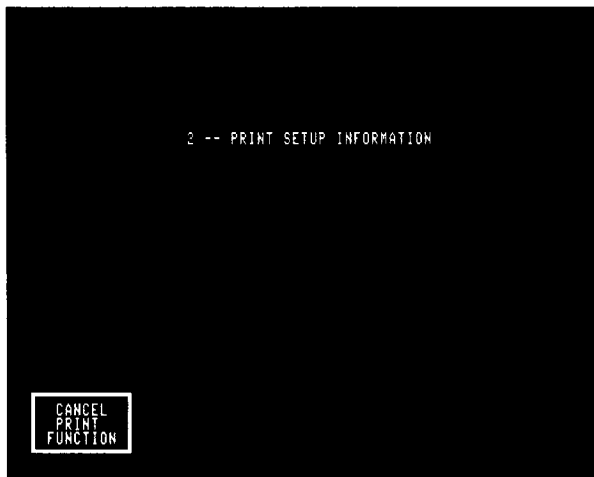
Figure 2-1. Print Setup Information menu with printer operating. This is a typical display during printing. The only action allowed the user is to stop printing using the CANCEL PRINT FUNCTION soft key or the STOP key. Text being printed will scroll through the blank section of the screen when the printer is operating.
